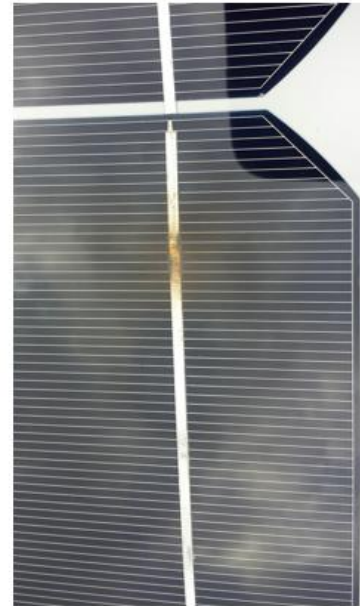
1 Solder bond failure of one cell interconnect
