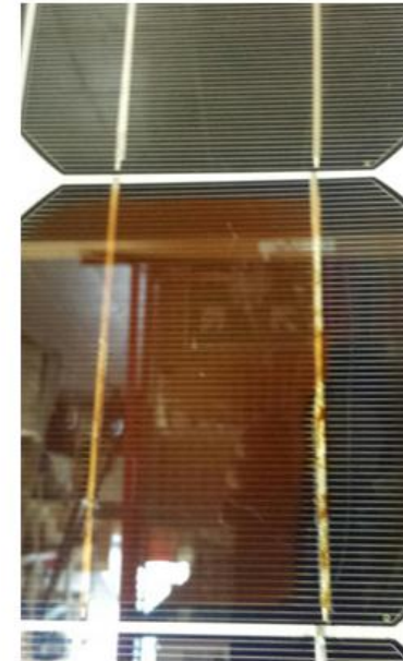
2 Solder bond failure of both cell interconnects
