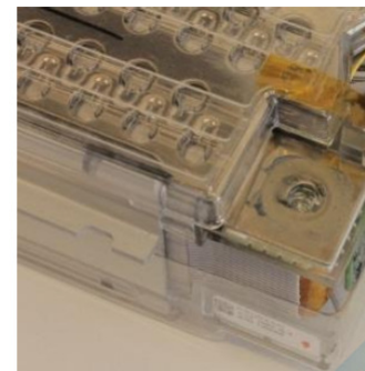
Aluminum side frame, plastic top/bottom cover
