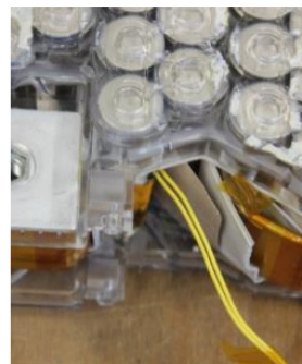
top plastic tray with glued module pole interface plate
